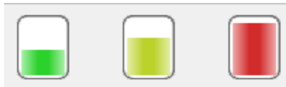
Example of the disk usage display. As more disk space is used to store messages, the icon changes from green (left), to yellow (middle), to red (right)
